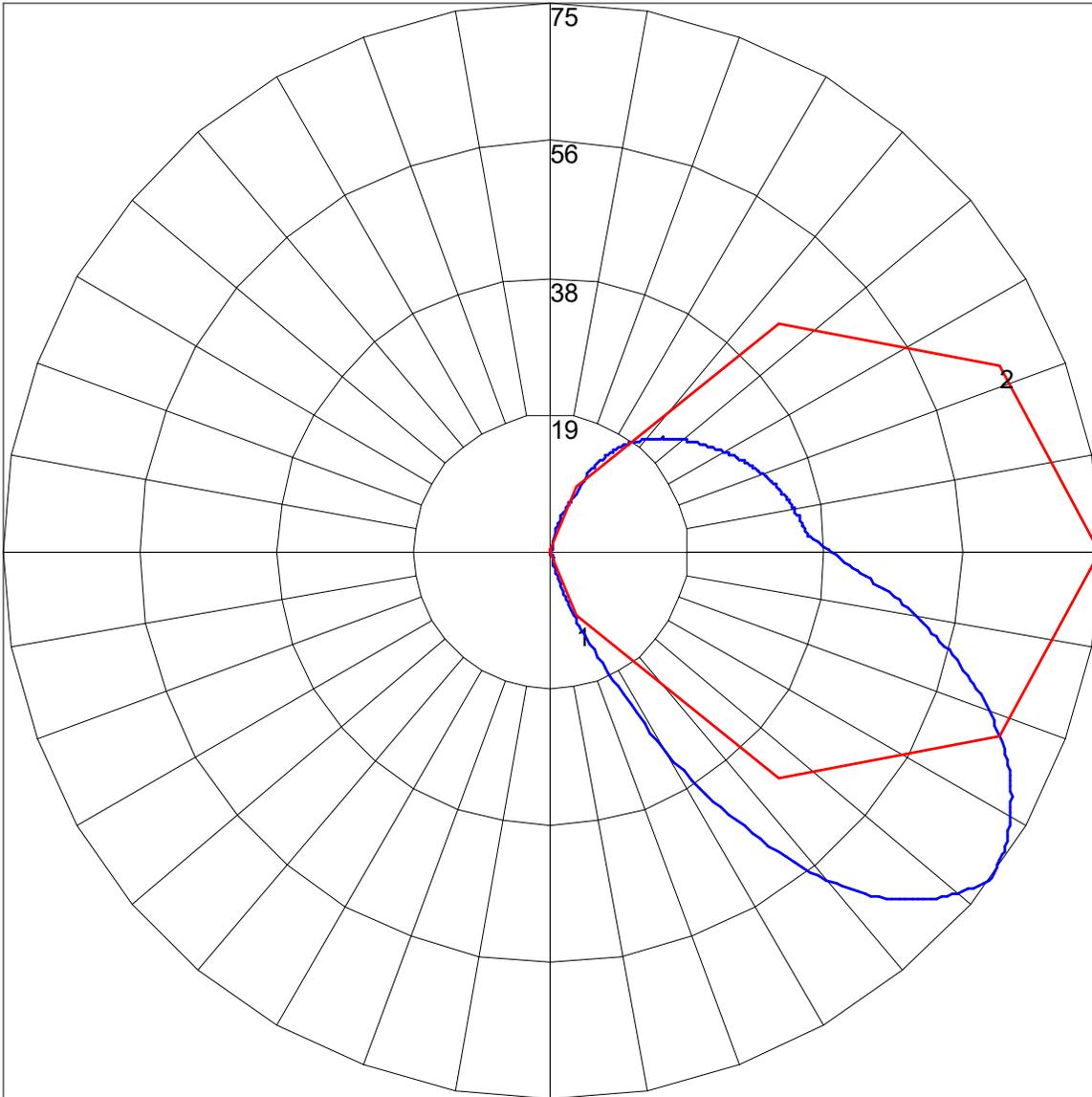
Maximum Candela = 75.02 Located At Horizontal Angle = 0, Vertical Angle = 53.5
