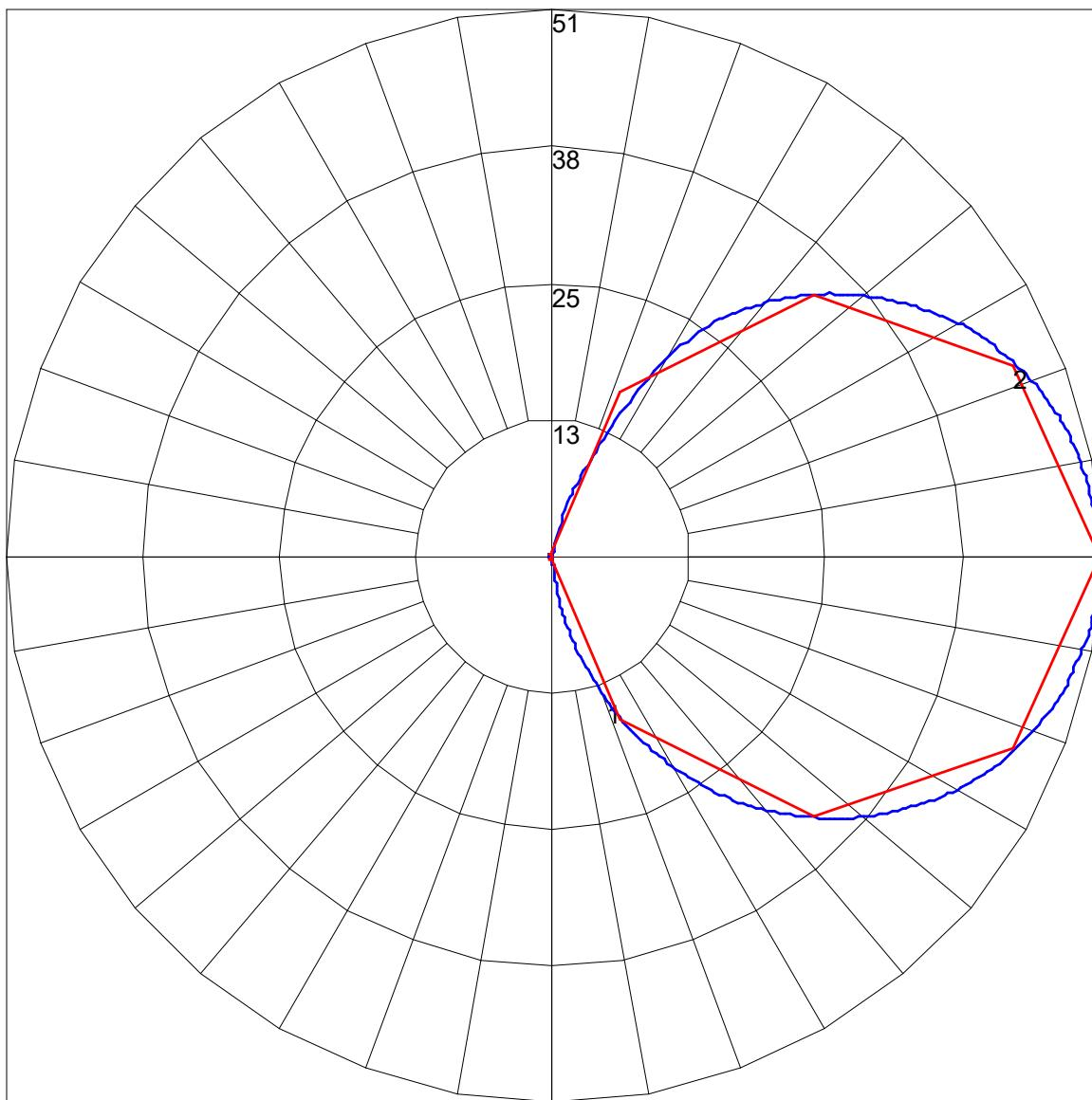
Maximum Candela = 50.86 Located At Horizontal Angle = 0, Vertical Angle = 91
