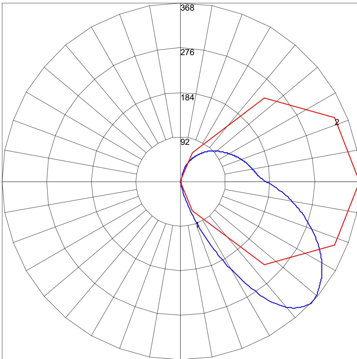
Maximum Candela = 368 Located At Horizontal Angle = 0, Vertical Angle = 47.5
