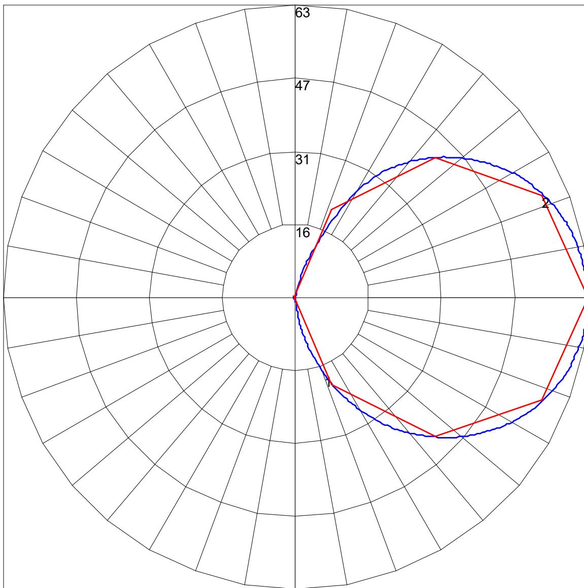
Maximum Candela = 62.79 Located At Horizontal Angle = 0, Vertical Angle = 91
